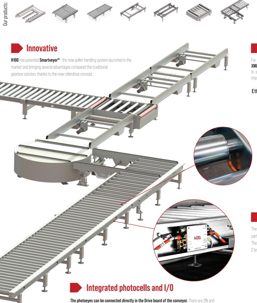
The photoeyes can be connected directly in the Drive board of the conveyor. There are 2IN and 1 programmable OUT for each Roller Drive. The drive board is able to manage up to 2 rollerdrives. The drive is equipped with plug-in connectors fast IP67, both for the power and supply section and for the photocells, there is also the unique MAC Address for easy system setup.
